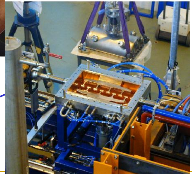
Rex-Isolde IH (CERN), 202.6 MHz
