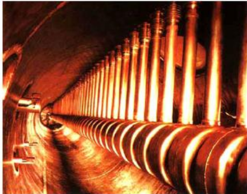
Saturne DTL (Saclay) : -> 20 MeV, 200 MHz
